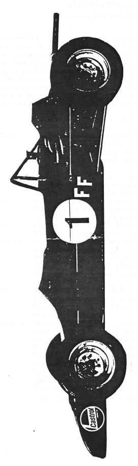
tall (6.5") drivers but incorporating the later "wedge" style body with its low drag factor. Owing to its having been specifically designed for Formula Ford, the WDF.2. attains a weight of 890 lbs. The WDF.2. is a refinement of our very successful WDF.1. model, retaining the ability to seat very
